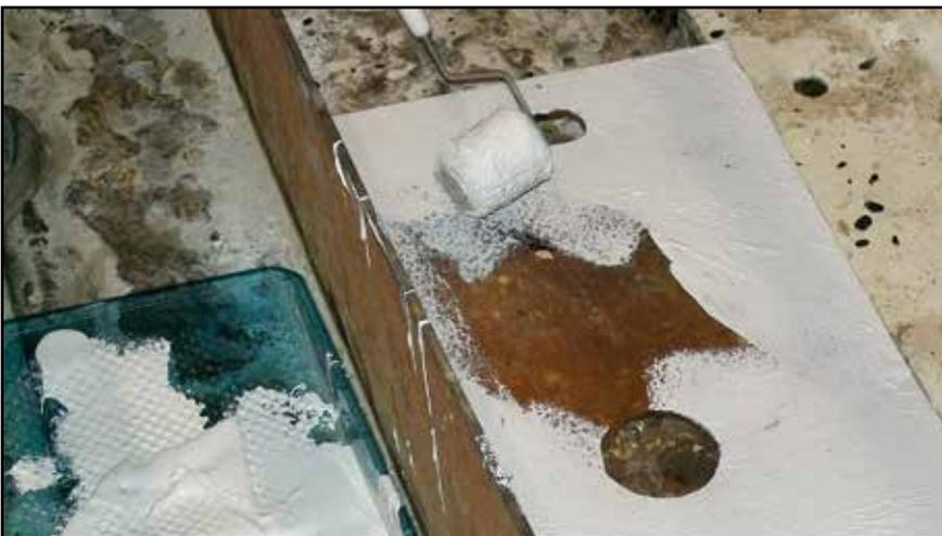
Exposed and rusty metal on the casting deck represents an extreme risk for molten metal explosion. Proper application of Wise Chem reduces the risk of serious personal injury and plant damage.
